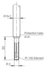
Sensor tip Ø 3 mm Halftime:  $t_{50} \le 0.5$  s 90% time:  $t_{90} \le 1.5$  s
