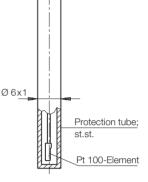
Sensor tip Ø 4 mm Halftime:  $t_{50} \le 2.4$  s 90% time:  $t_{90} \le 6.5$  s
