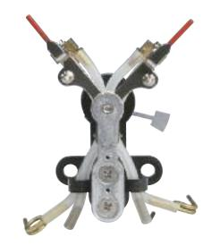
Pneumatic limit signal transmitters work without contact and with a very low feedback onto the mechanical pressure measuring system. They do not generate any electrical contact problems like wear, welding or excessive contact transfer resistance. Pneumatic contacts are used where controls work using pneumatic regulation and require high reliability and switching frequency, i.e. a longer life.
