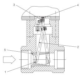
When the diaphragm plate is moved by the flow in the flow direction, the lever arm is deflected by the force of the leaf spring.
