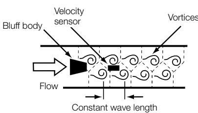
The measuring principle is based on the Karman vortex street. A specially shaped bluff body is located in direction of the flow. From a certain flow velocity on vortices are generated through the bluff body.
