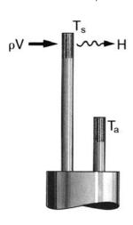
Energy is transferred to the flowing medium - causing increased current flow through the sensor. The electrical energy required to maintain the sensor at a constant temperature is proportional to the mass flow of the gas.
