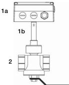
The ball valve assembly allows for the exact alignment of the sensing head within seconds during instalment and removal, with only interrupting the process flow for a short moment. The ball valve assembly is suitable for pressures up to 16 bar (PN16) and available for pipe diameters DN15 ( $\frac{1}{2}$ ") to DN50 (2"). During installation in the pipeline, observe the required inlet and outlet paths as given in the operating instructions.
