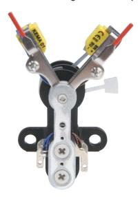
The inductive contact device comprises mainly the control head (initiator) attached to the setpoint pointer with its completely assembled encapsulated electronics and mechanical assembly with moving control vane. The control vane is moved by the instrument pointer (setpoint pointer). The control head is supplied with DC voltage.
