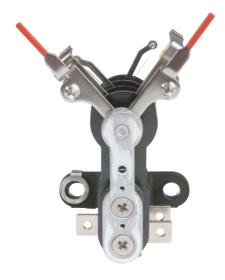
These contacting devices switch free of delay in the same way as the motion of the actual-value pointer. They should be used where no contact loading is required and the instruments are not exposed to vibrations. Due to sparking the contacting devices should not be used where there is a danger of explosion. Care should also be taken that the contacting devices are not exposed to the effects of aggressive vapours.
