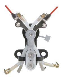
Pneumatic limit signal transmitters work without contact and with a very low feedback onto the mechanical pressure measuring system. They do not generate any electrical contact problems like wear, welding or excessive contact transfer resistance. Pneumatic contacts are used where controls work using pneumatic regulation and require high reliability and switching frequency, i.e. a longer life.
