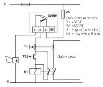
equipment such as contactors or relays of the external interlock circuit correspond to VDE 0660 or VDE 0435 respectively.
