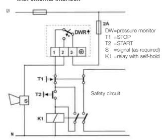
When the interlock circuit shown above is used, the requirements in accordance with DIN 57 116/VDE 0116 are fulfilled if the electrical
