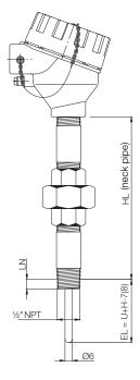
U = immersion length thermowell (see drawing thermowell)
